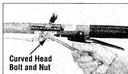
Photo 2-20: Attach Kohler engine throttle lever to handlebar.
