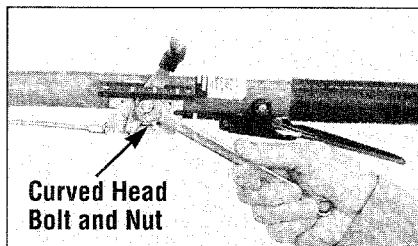
Photo 2-20: Attach Kohler engine throttle lever to handlebar.
