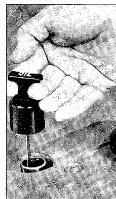
Photo 2-19: Remove 8HP Kohler engine dipstick to add motor oil.
