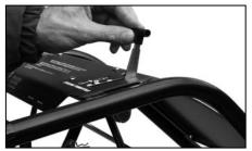
Figure 3-8: Engine Throttle Lever.
