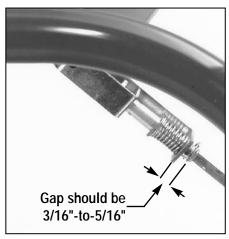
Figure 2-9: While squeezing Forward Clutch paddle, measure gap between end of bracket and E-ring.
