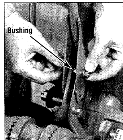
Photo 2-10. Insert bushing, then install bolt through upper hole in lever and yoke plates. Loosely add the star washer and the hex nut.
