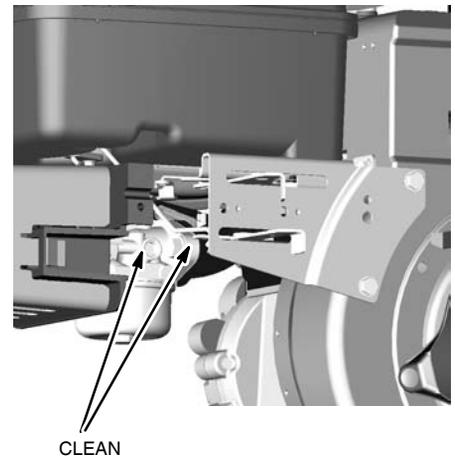
**Muffler, Spark Arrester**
