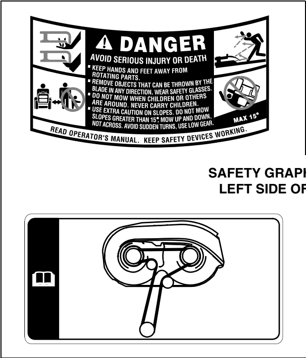
INFORMATION GRAPHIC – BELT ROUTING LOCATED ON LEFT SIDE OF MOWER DECK
