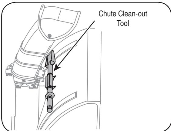
A chute clean-out tool is fastened to the top of the auger housing with a mounting clip. The tool is designed to clear a chute assembly of ice and snow.
