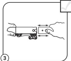
3 Remove cap from lower boom. Push cutting attachment into coupler. Turn coupler knob clockwise to tighten.
