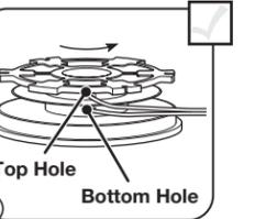
4 Insert the end of one line into the top hole and the end of the other line into the bottom hole.
