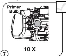
7 Press primer bulb 10 times, or until fuel is visible
