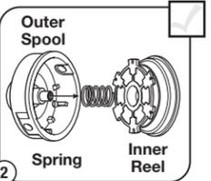
2 Remove the inner reel and spring.
