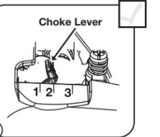
12 Move choke lever to Position 2 and squeeze throttle.
