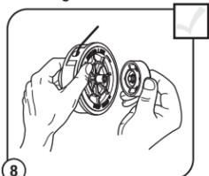
8 Hold the inner reel and outer spool together. Firmly pull the two line ends to release them from the holding slots. Screw the bump knob on clockwise. Tighten the bump knob securely.
