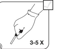
13 Pull rope 3-5 times to start engine. Run unit for 30-60 seconds to warm up.
