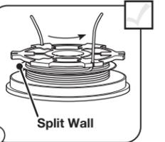
5 Wind the line tightly in the direction shown on the inner reel. The split wall will divide the line. Wind the line until it is completely divided and about 6 inches (150 mm) of line remains.
