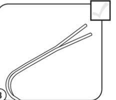
3 Cut one 6-foot (1.8 m) length of new 0.095" split line trimming line. Split each end about 6 inches (150 mm).
