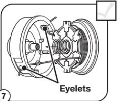
7 Pass the two line ends through the eyelets. Place the spring inside the inner reel. Insert the inner reel into the outer spool. Push the inner reel and outer spool together.
