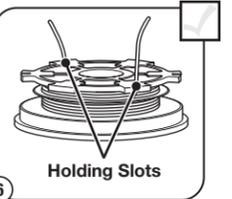
6 Insert the two 6-inch sections into the two .095 holding slots.
