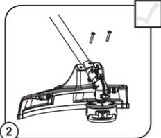
2 Place shield onto mount bracket. Securely screw 2 shield screws through holes on mount bracket and into shield. Make sure screws are tightened equally so there is an equal gap between bracket and shield on each side.
