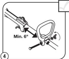
4 Put D-handle on shaft. Move handle a minimum 6 inches away from shaft grip. Insert clamp bolt and tighten the wing nut.
