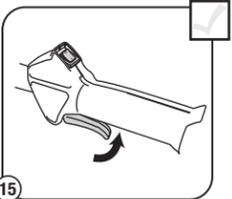
15 Continue to squeeze throttle. Run unit for an additional 60 seconds to complete warm-up. Unit may be used during this time.
