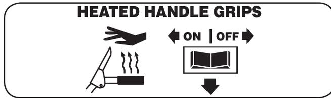
This switch is located on the rear of the snow thrower dash panel. To activate the heated handles, toggle the switch to the "ON" position to generate heat within the handle grips. Toggle the switch to the "OFF" position after using the snow thrower.
