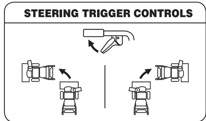
The left and right wheel steering trigger controls are located on the underside of the handles.
