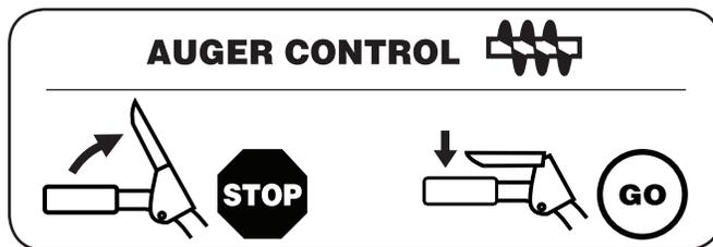
The auger control is located on the left handle. Squeeze the control grip against the handle to engage the augers and start snow throwing action. Release to stop.
