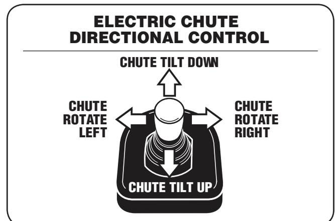
The electric chute directional control is located on the right side of the dash panel.
