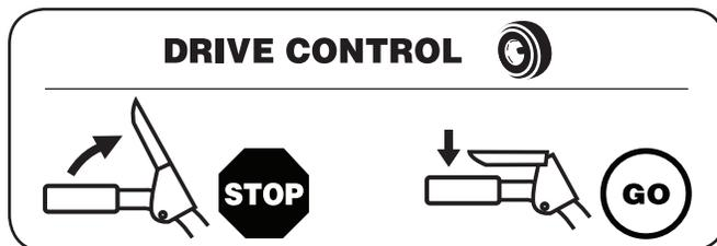
The drive control is located on the right handle. Squeeze the control grip against the handle to engage the wheel drive. Release to stop.
