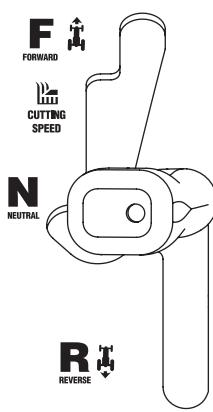
When mowing, place the speed control lever in the "Cutting Speed" position, or a slower forward speed for the best results.
