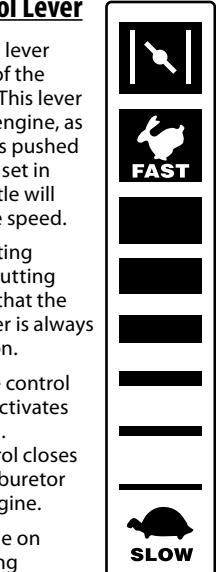
When mowing, place the speed control lever in the "Cutting Speed" position, or a slower forward speed for the best results.
