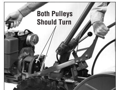
Figure 5-26: Checking Reverse Disc in REVERSE.
