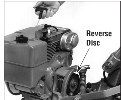
Figure 5-25: Checking Reverse Disc in NEUTRAL.
