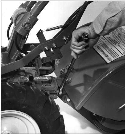
Figure 4-24: Loosening attachment swing-bolts.
