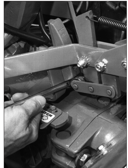
Figure 5-13: Insert slotted end of belt adjustment tool between roller and bracket, with the flat side of the slotted end facing the roller.
