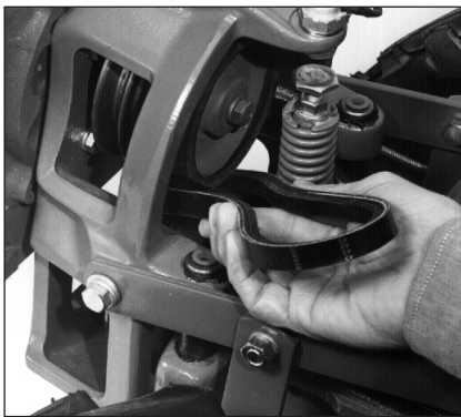
Figure 5-20: Shift into FORWARD and remove the belt.
