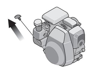
Pull starter rope with quick, full arm stroke.
