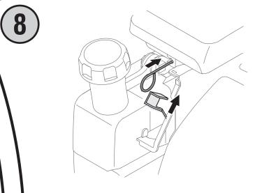
Slide choke lever to full choke position and place throttle in rabbit (fast) position.
