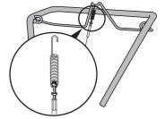
Thread end of cable onto screw attached to control lever. Refer to manual to adjust tension *before* tightening jam nut.
