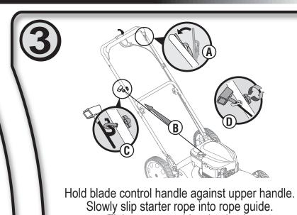
Tighten rope guide wing knob.
