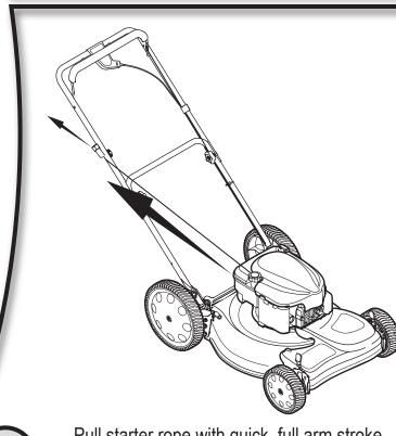
Pull starter rope with quick, full arm stroke.
