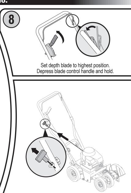
Pull starter rope with quick, full arm stroke.
