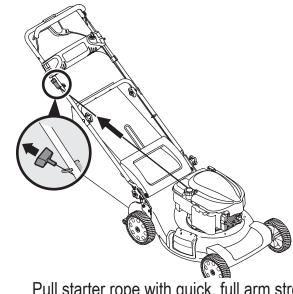
Pull starter rope with quick, full arm stroke.
