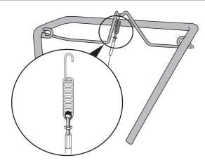
Thread end of cable onto screw attached to clutch bail. Refer to manual to adjust tension **before** tightening jam nut.
