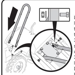
Loosely attach lower handle to frame using the 3/8"-16 x 3/4" hex head screws, flat washers, and 3/8"-16 hex lock nuts.
