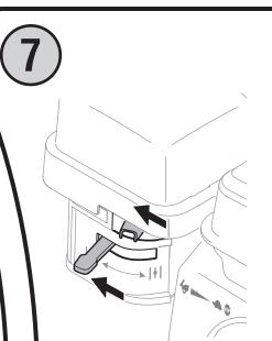
Move choke control to full choke position.
