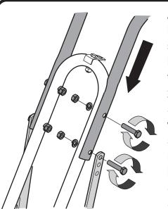
Attach upper handle and handle support brackets to lower handle using the 5/16"-18 x 1-1/2" screws, 5/16" split lock washers, and 5/16"-18 hex nuts. Tighten all hardware in Step 1 and Step 2.
