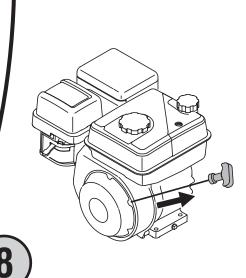
Pull starter rope with quick, full arm stroke. It may take more than one pull to start cold engine. Once started, slowly move choke control to off (run) position.
