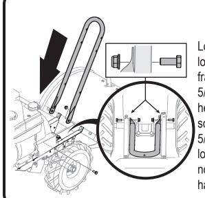
Loosely attach lower handle to frame using the 5/16-18 x .75 hex head cap screws and 5/16-18 flange lock nuts. Do not tighten hardware.
