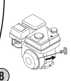
Pull starter rope with quick, full arm stroke. It may take more than one pull to start cold engine. Once started, slowly move choke control to off (run) position.
