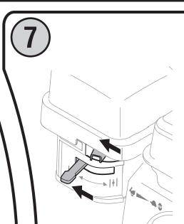
Move choke control to full choke position.
