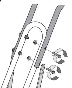
Attach upper handle and handle support brackets to lower handle using the 5/16-18 x 1.50 screws and 5/16-18 flange lock nuts. Tighten all hardware in Step 1 and Step 2.
