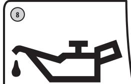
Pour the entire contents of the SAE 10W 30 oil bottle (supplied) into the oil fill. Check the oil level by inserting the dipstick (not threading it) into the oil fill. (Refer to the Operator's Manual)
