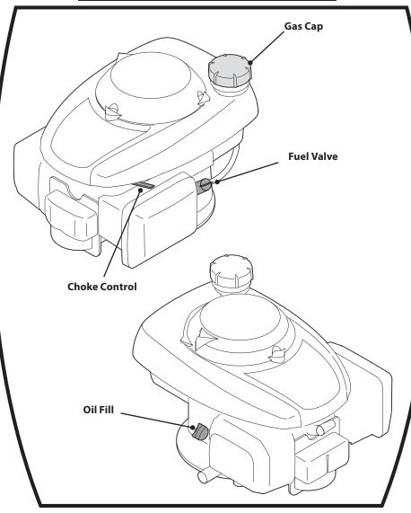
Rotate the fuel valve into the Open position. Move the choke control into the Choke position.
