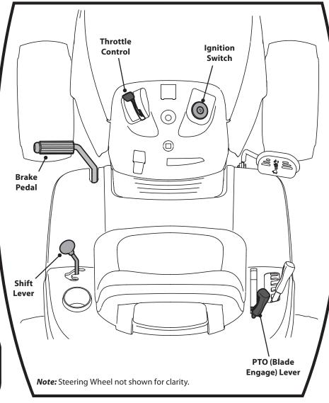
Move the throttle control into the Choke position
