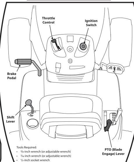
1. With the wheels of the tractor pointing straight forward, place the steering wheel over the steering shaft. 2. Secure the steering wheel with the washer (cupped side down) and hex bolt. 3. Push the steering wheel cap
