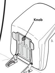
Slide the seat rearward and align the center mounting hole in the seat with the slot in the seat pan and secure the seat with the knob.
