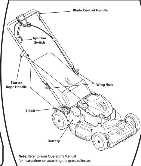
A. Insert the T-bolts removed in Step 1B through the handle brackets to secure the handle in place.
