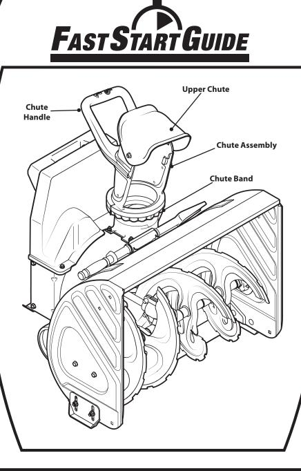
Gip the discharge chute handle onto the discharge chute, as shown in the figure below.
