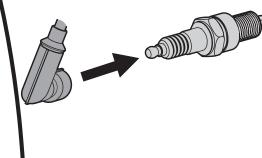
Make sure the spark plug boot is connected to the spark plug before attempting to start.
