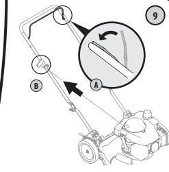
While standing behind the machine, pivot the Blade Control Handle against the premium drive control.
