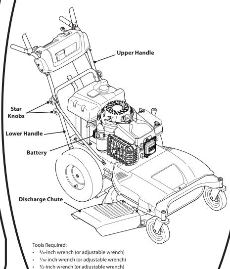
Remove the lower star knobs and carriage screws from the lower handle.
