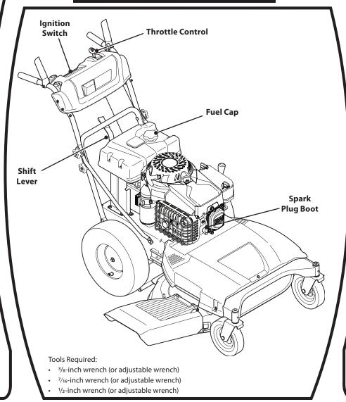
Fill fuel tank with clean, fresh gasoline. Do not fill above the base of fuel tank neck.
