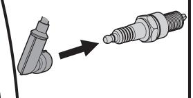
Make sure the spark plug boot is connected to the spark plug before attempting to start.
