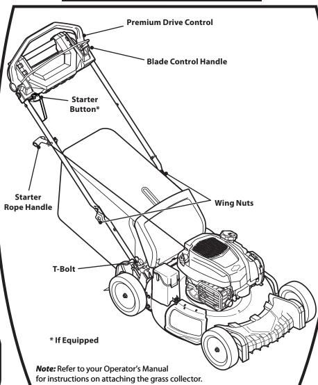
Insert the T-bolts removed in Step 1B through the handle brackets to secure the handle in place.
