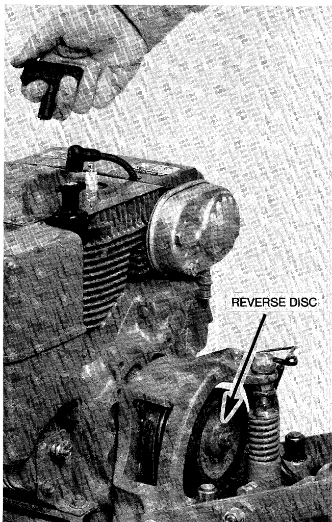
6-34: With shift lever in "NEUTRAL", only the reverse disc should turn.
