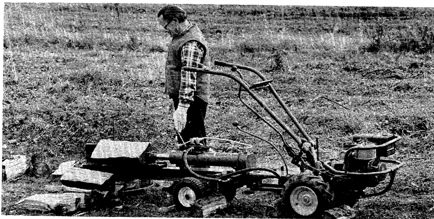
9-11: The Log Splitter produces 13 tons of hydraulic pressure.
