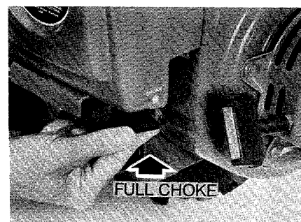
2-12: Choke control on 8 HP Engine.
