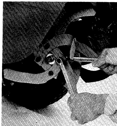
6-41: Removing a single tine.
