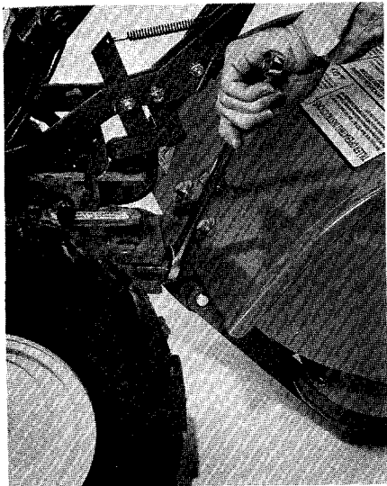
5-9: Tighten both swing-bolts.
