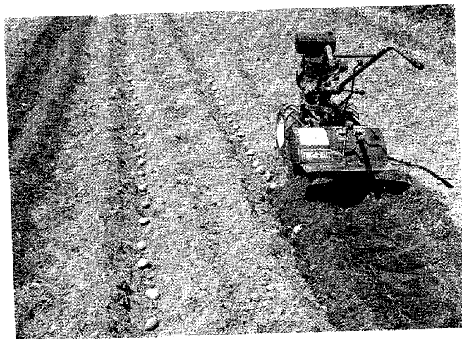
(Photo 6/35) When seed potatoes are in the ground, the labor saving Hiller wings will bury them. As potatoes grow, hill them as needed.
