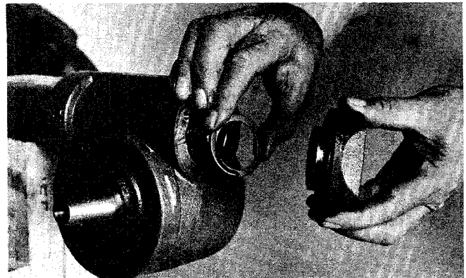
(Photo 8/37) Shims remove play in shaft.
