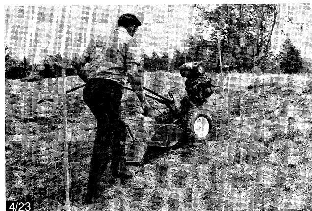
The powered wheels will pull the tiller up the hill and will also hold the tiller back while you go downhill to prevent the tiller from going too fast.
