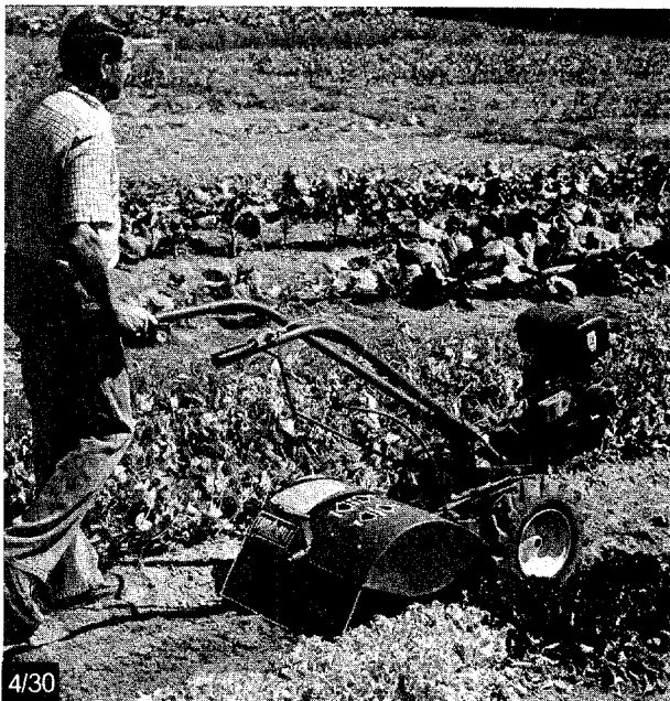
4/30 Avoid deep cultivation that can sever shallow plant roots. Set your depth regulator to till at a depth of 1½ to 2 inches.
