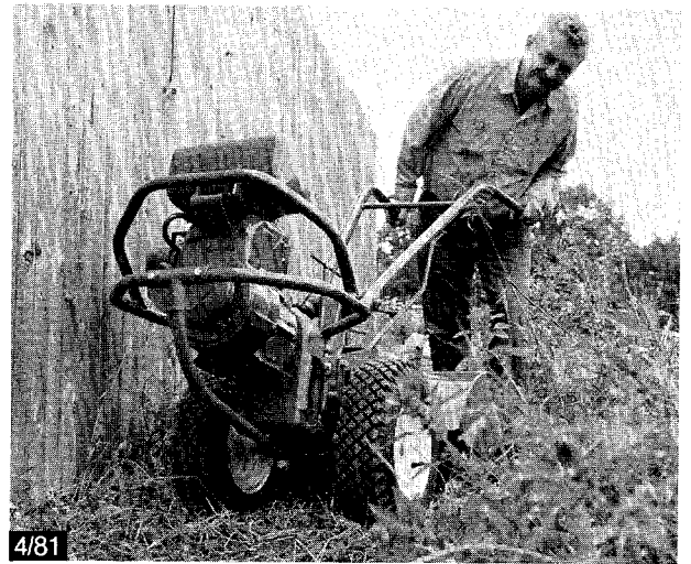
Protects carburetor and engine from bumps and scrapes.
