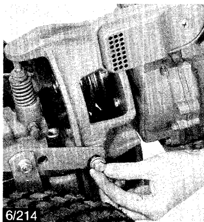
Fasten yoke to engine mount.
