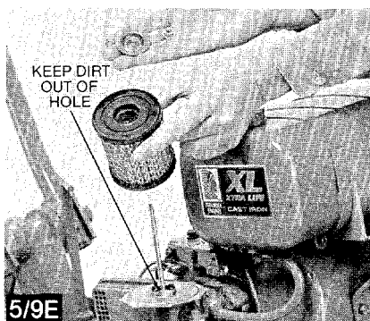
5/9E Remove 7HP paper element.
