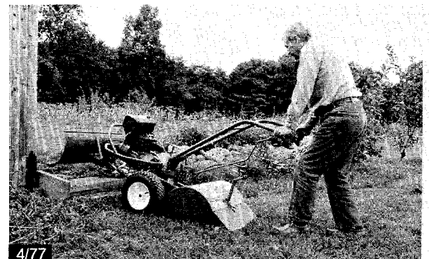
4/77 Tine removal is not only safer, it permits you to raise the front higher, and the blade banks easier.
