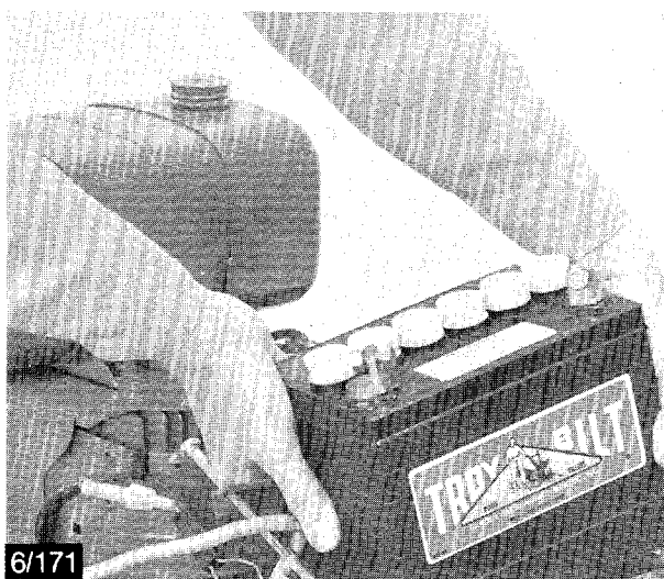
Remove battery from tiller.
