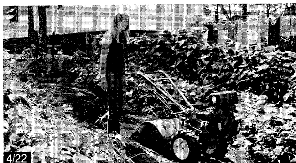
Tilling vertically on a slope allows you to walk alongside the tiller guiding it with one hand.
