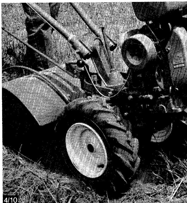
Bar Tread Tires can make the difference in loose soil
