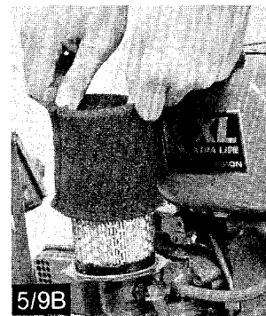
5/9B Remove foam element.
