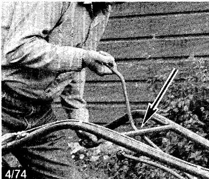
4/74 If lever hits handlebar cross-piece, switch ratchets as shown in Photo 4/75.
