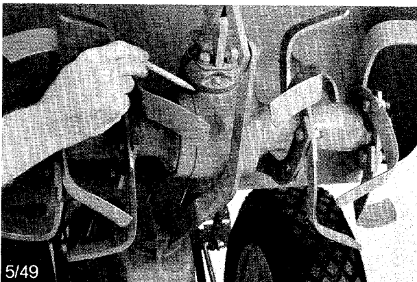
Look for oil leak where end cap joins tiller housing.
