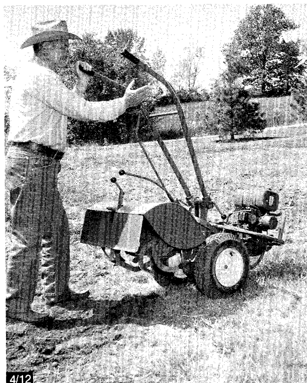
Operating tiller in reverse will usually untangle debris.
