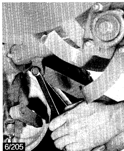
Attach drag bar to tab on tube.
