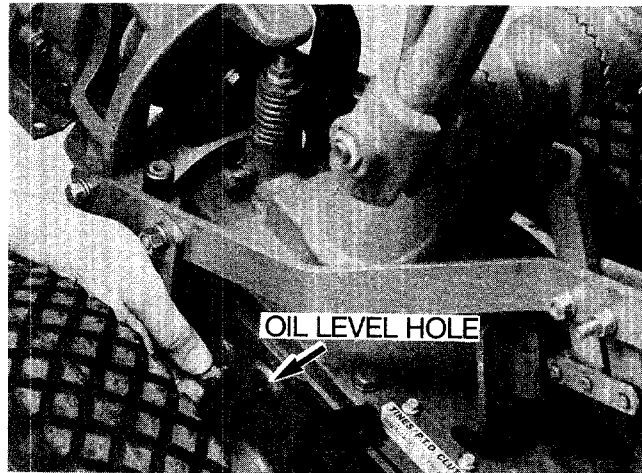
1/10—Remove oil level check plug from left side of Power Unit Transmission.
