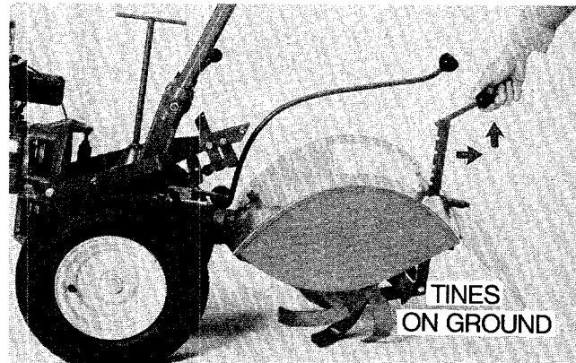
1/9—Pull Depth Regulator Lever back and up to lower tines.
