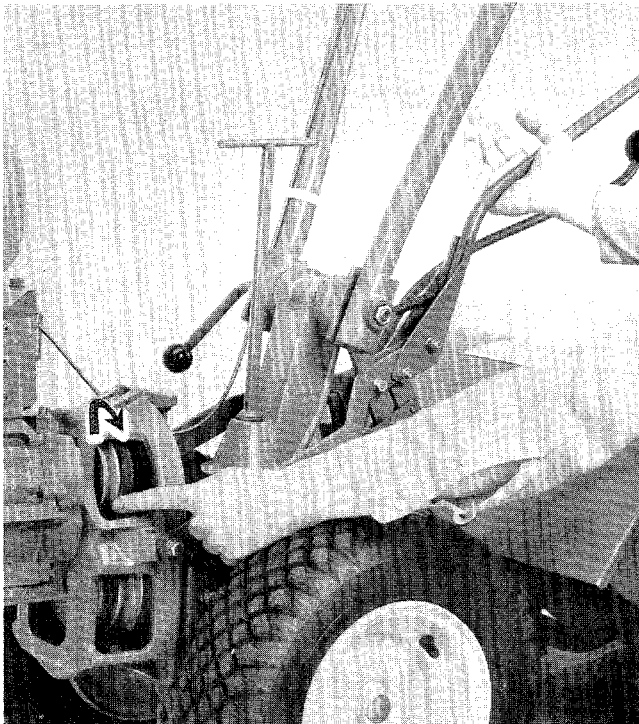
3/27 —With lever in Reverse, move belt on upper pulley into groove furthest away from engine.
