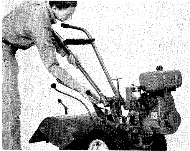
3/18 —Loosen adjustment stud to raise handlebars up or down.
