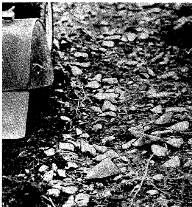
5/22—In rocky soil, use slower wheel and tine speeds. Get rid of stones that are larger than baseballs; let the smaller ones stay.
