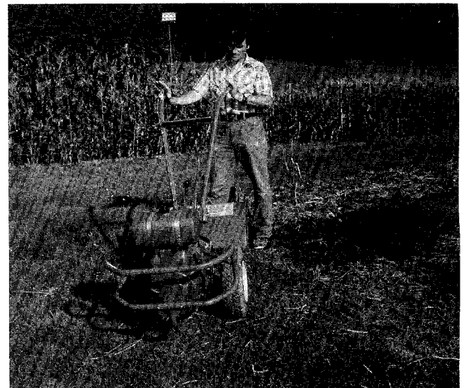
5/9—Lift and push handlebars to turn tiller.
