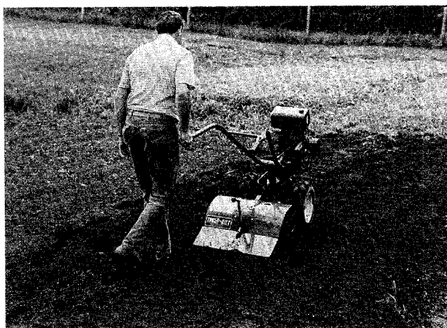
5/17 —The final seedbed should be tilled 6 to 8 inches deep.
