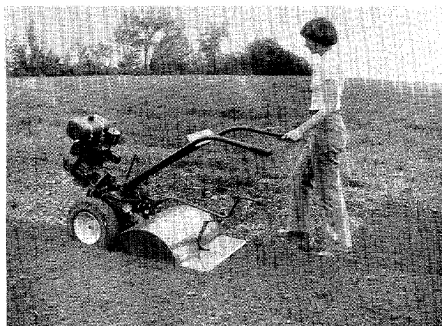
5/12—Begin tilling shallow and work down gradually deeper with each pass.
