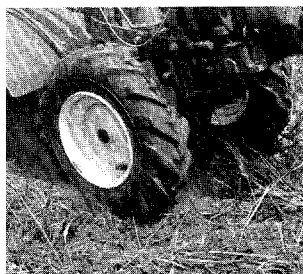
5/14—Bar Tread Tires can make the difference in loose soil.
