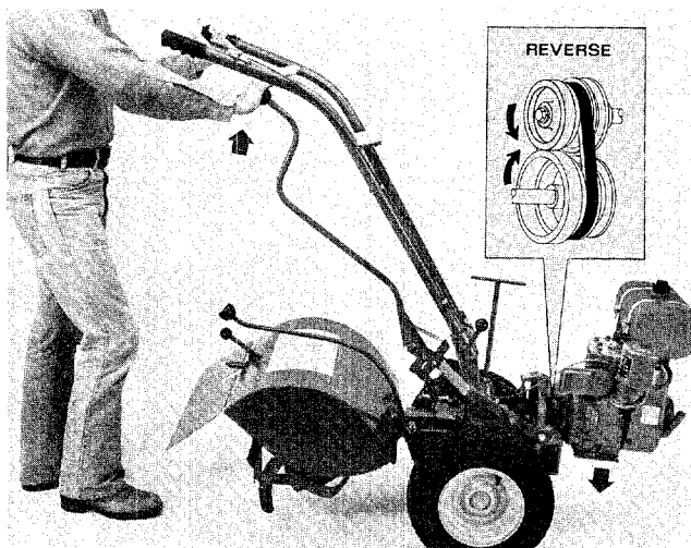
6/23—In Reverse, rubber disc drives transmission pulley.
