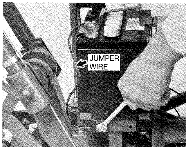
7/71—Replace negative cable with jumper wire.
