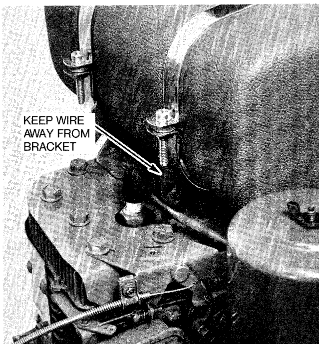
7/82—Check condition of spark plug and wire.
