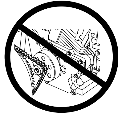
Figure 1. DO NOT use Without Engine Shaft Guard
